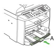
To load Legal-size paper, leave the front panel of paper cassette open and adjust the paper guide rail (A) for Legal-size paper.
